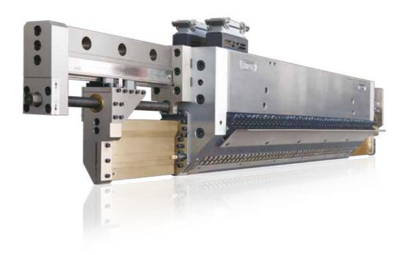
Jwell Company's high-speed film coating die adopt T-type thick edge with manual adjustment system to simplify the product width switching operation and online adjusting. Each independent edge adjusting system can minimize the thick edge issues. Thus effectively reducing the waste of the polymer and the substrate. This dies suitable for the produce the width below 5000mm, thickness of 0.012–0.12mm of PP, PE, PET, EVA coating products.
